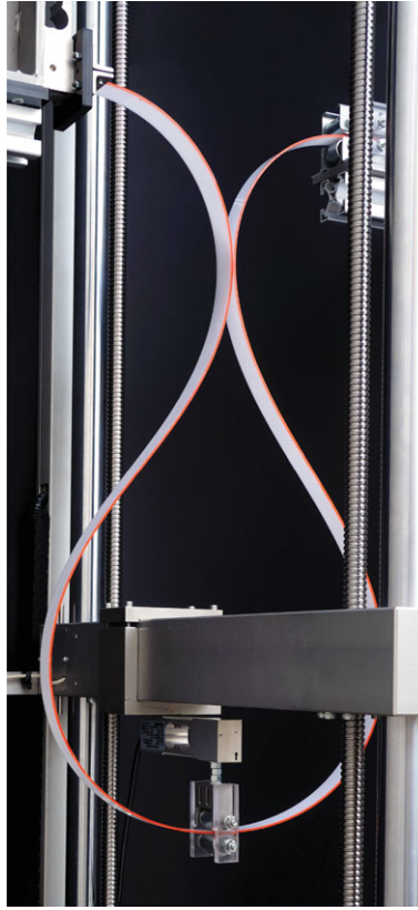
Figure 8. A photo taken at the dripping point during a quasi-static experiment. A symmetry breaking has occurred, although it is not particularly evident.
