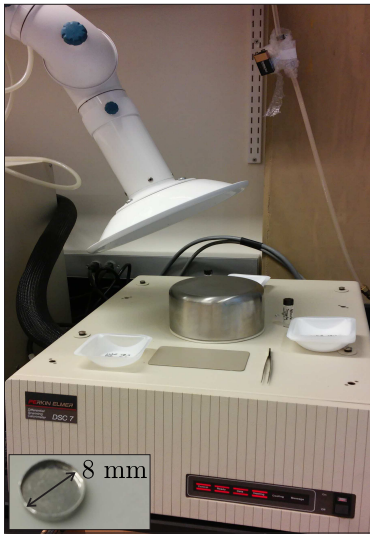
Figure 5. Left: Differential Scanning Calorimeter (DSC) employed in the resin cure kinetic modeling; the aluminum hermetic DSC pan containing 7-10 mg of resin is shown in the inset. Right: specific heat flow \bar{\Phi} = \Phi/w as a function of temperature during a DSC dynamic thermal scan performed at 10^\circ\text{C}/\text{min} for an uncured sample. The glass transition temperature is at 53.09^\circ\text{C} , while the exothermic peak occurs at 143.37^\circ\text{C} . The dashed black line represents the baseline, necessary to calculate the amount of heat generated during cross-linking.
